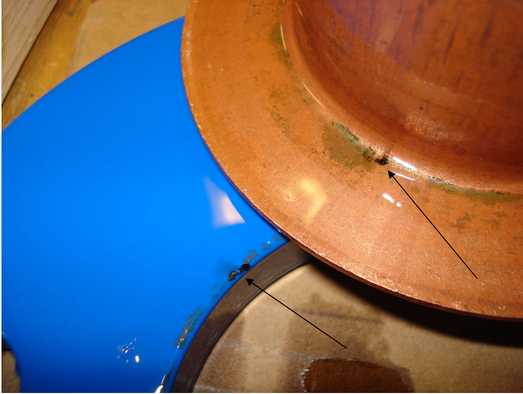
Without 'electrolysis insulator'
